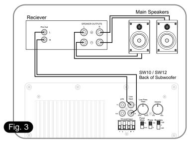
Amps and receivers with Pre-Out jacks: connect the SW10II OR SW12 from the Pre-Out into the SW10II OR SW12's Line Input.
